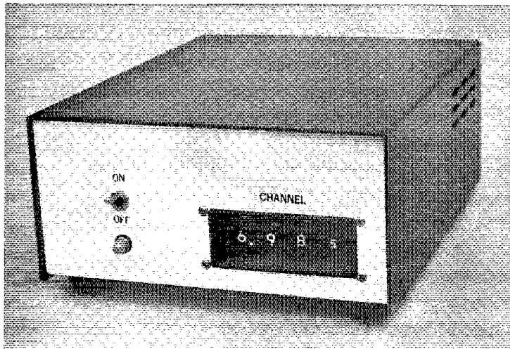
An ON-OFF switch and the frequency-selector switches are the only controls mounted on the front panel of the synthesized 2-meter transmitter. A microphone connector and accessory plug are located on the rear panel.
