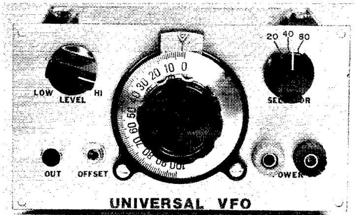
Exterior view of the completed 3-band VFO. Double-sided pc board material is used for the panel and box walls in this version by Circuit Board Specialists.
