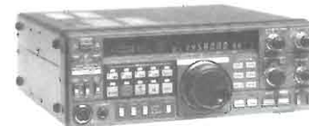
TS 711 E/DCS VHF 144-146 MHz TS 811 E/DCS UHF 430-440 MHz 2 m, 25 W, All Mode base. 70 cm, 25 W, All Mode base.
